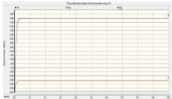
Fig. 12. active power at buses 1, 10, 33 of IEEE 33 bus distributed system without DG penetration at bus 10.
