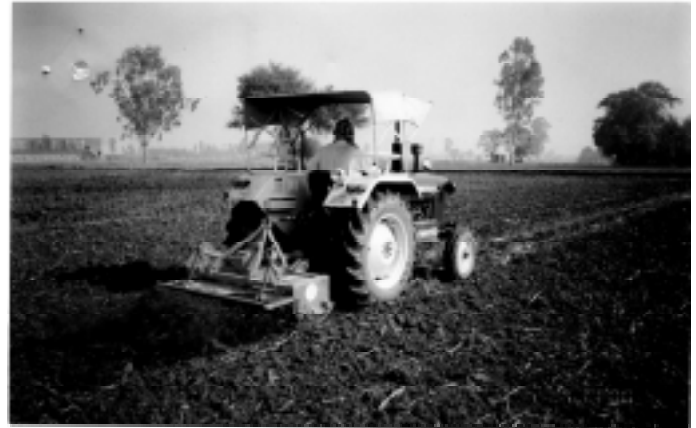
Figure 2 A view of tractor operated rotavator while preparing the field for wheat sowing with shield in the raised position
