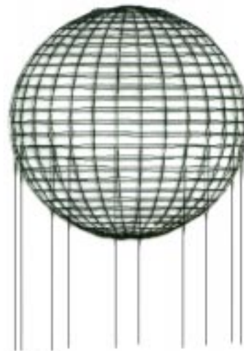
Figure 4 First mode shape with buckling load factors
