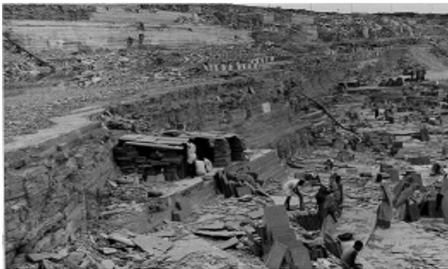
Fig. 1: Conventional Manual Mining of Kotah Stone
