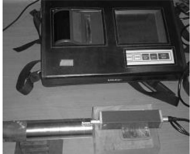
Fig. 3: Mitutoyo Surface Tester
