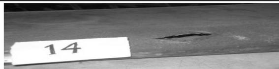
**Sample No. MRH—14** - Both the outer and inner surface shows uniform scale deposit, mixture of black and brown color. The neighboring surface of leakage shows minor bulging effect.
