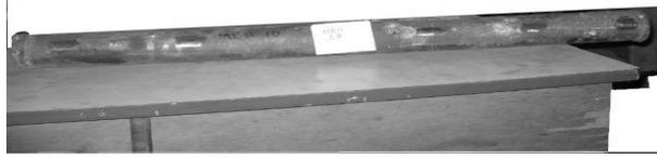
**Sample No. MRH—12** - Both the outer & inner surface shows uniform scale deposit, mixture of black & brown color. The neighboring surface of leakage shows minor bulging effect. Thinning observed on the leakage spot.
