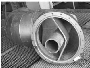
Fig. 8: Coal Pipe Bend with Mini Oil Gun Pipe
