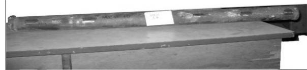
**Sample No. MRH—10** - Outer & inner surface shows uniform scale deposit, mixture of black and brown colour. The neighboring surface of leakage shows inverse bulging effect. Thinning observed on the leakage spot.
