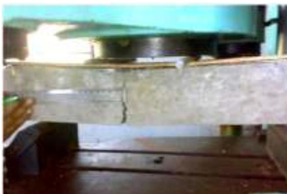
**Figure 10** Flexural strength test
