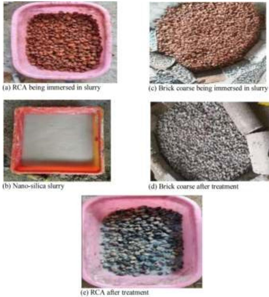
**Figure 3** Pre-soaking in nano-silica slurry for recycled aggregate and brick aggregate
