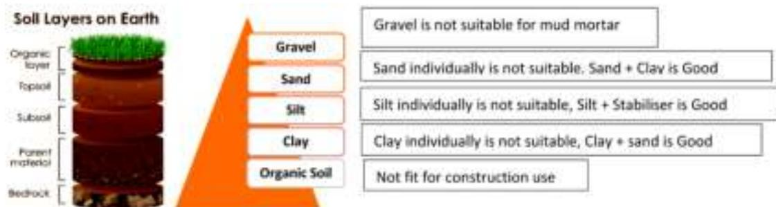
**Figure 3** The soil layers on earth (source: Freepik), the mud mortar combination (source: Laurie Baker Mud, [28])
