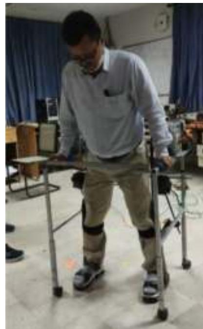
Figure 13 Final prototype of hip-knee exoskeleton
