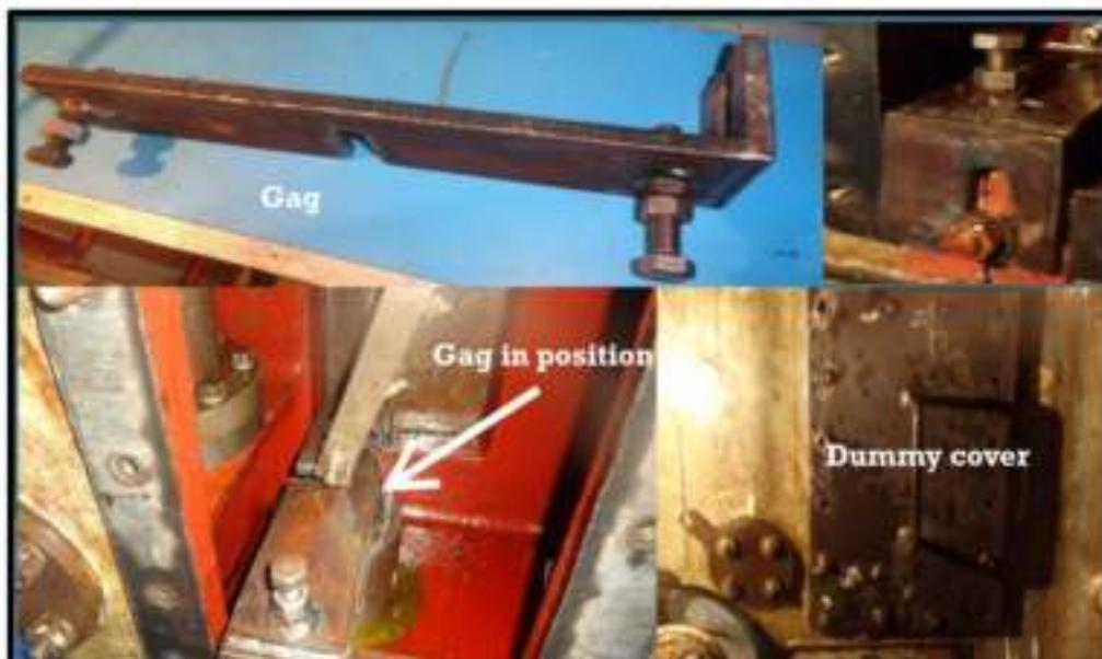
**Figure 3** Fabricated gag to arrest the movement of pilot valve plunger and FME dummy cover
