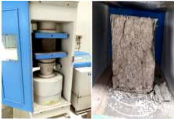
Figure 1 Compression test
