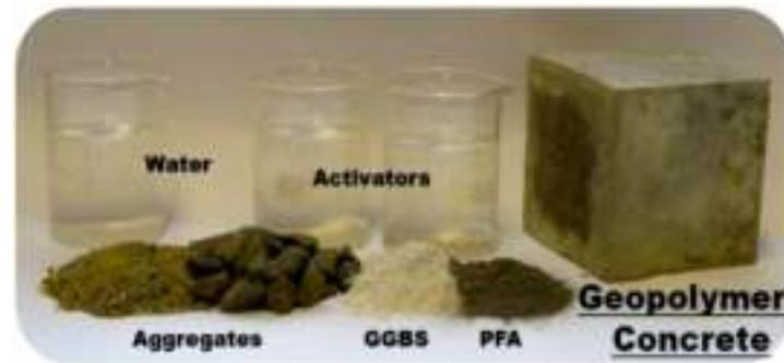
Figure 1 Geopolymer concrete
