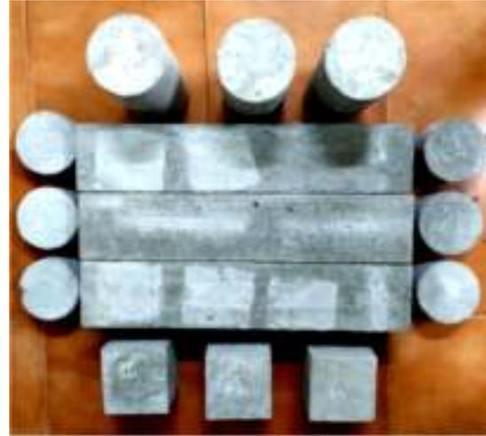
**Figure 3** Typical concrete specimens
