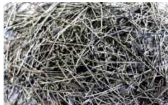
**Figure 7** Steel fibres
