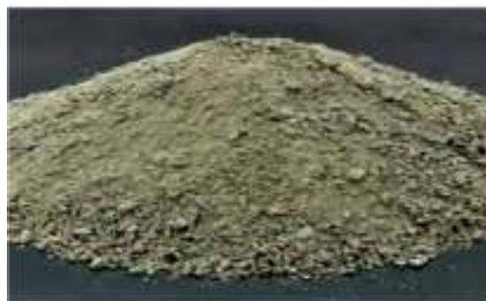
Figure 5 Manufactured sand (M.sand)
