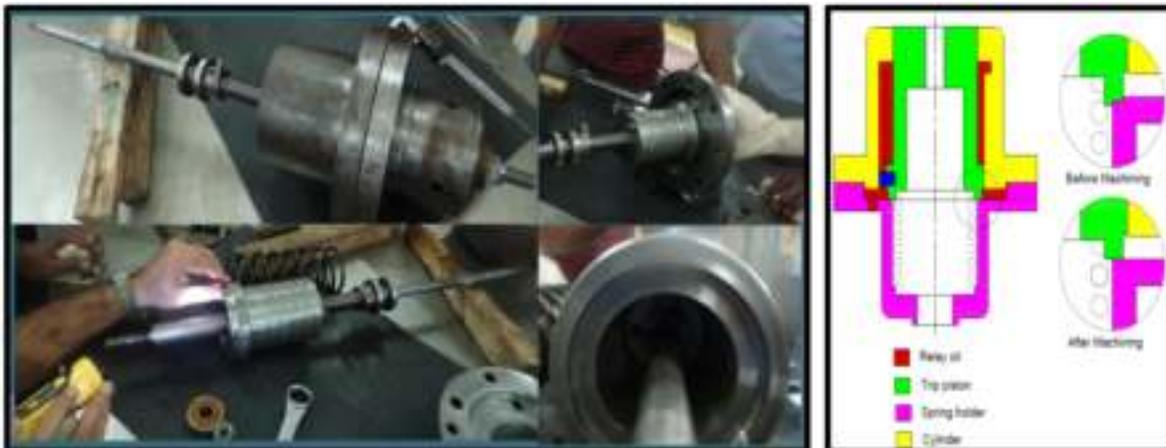
**Figure 4** Lapping (step) marks observed on the mating surfaces of trip piston and spring holder
