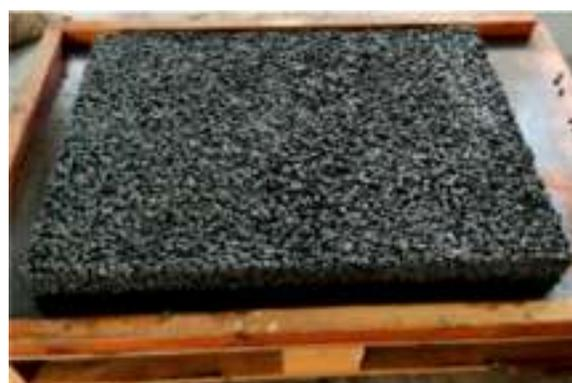
**Figure 2** Pervious concrete
