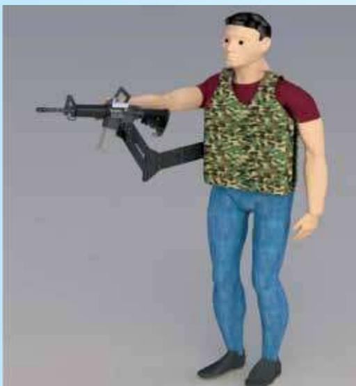
Final perspective rendered view of soldier wearing carbon fibre frame with the help of armour
