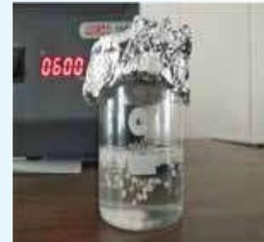
Dissolving polymer into the solvent
