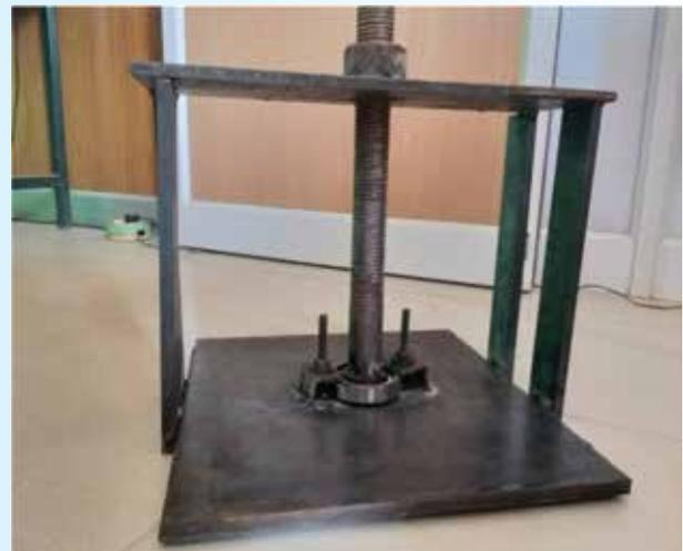
Compact book press compression mould setup used to fabricate the proposed hybrid composite
