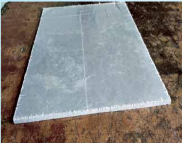
Fabricated hybrid fiber laminate
