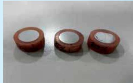
Sample prepared for hardness test
