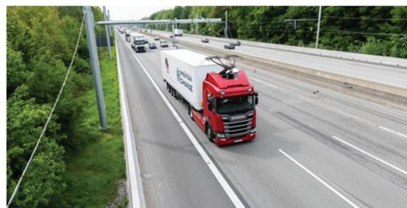
**Fig. 22** : E-Highway for intercity trucks and buses
