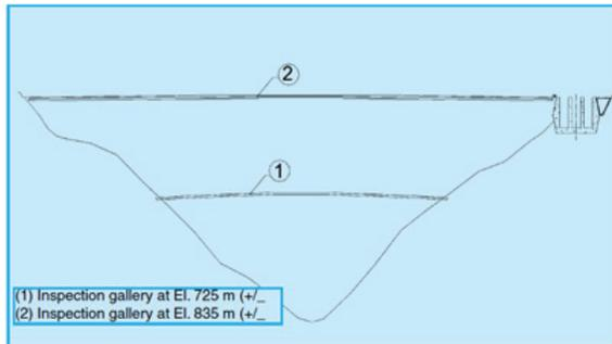
Figure: Longitudinal Section showing the Upper and middle level galleries in the core portion
