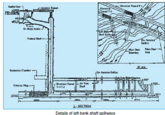
Details of left bank shaft spillways
