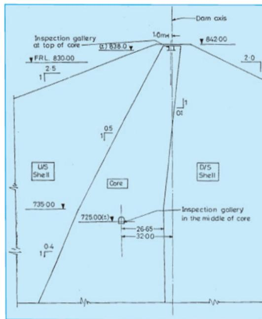
Figure: Mid-level Inspection gallery & Top Level Inspection Gallery in Dam Section
