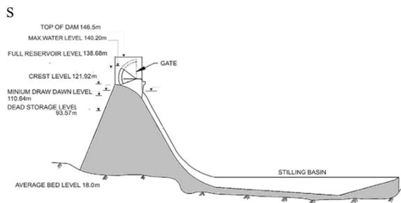
Figure: Cross-sectional view of the Sardar Sarovar Dam
