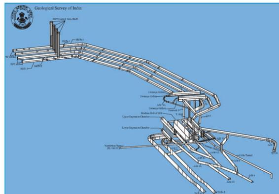
Figure: The model perspective projection of the entire power house
