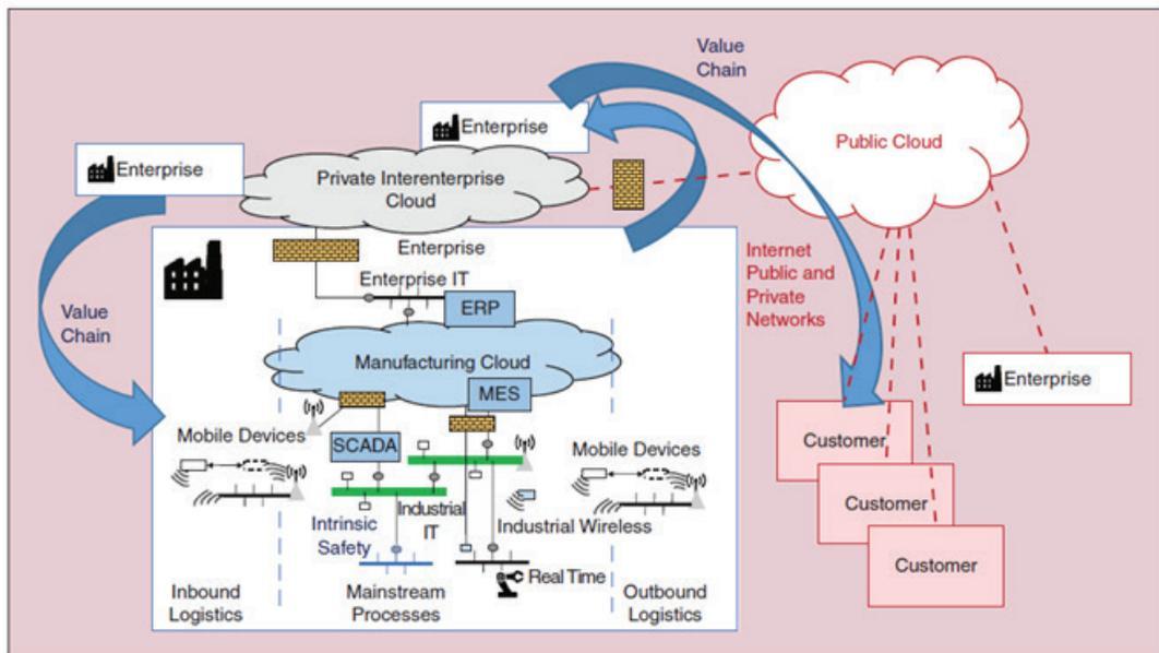
**Fig. 3** : The complexity of communication in industrial automation system (Mar Tin WollschLaeger et al, 2017), MES: Manufacturing Execution System, SCADA: Supervisory Control and Data Acquisition, ERP: Enterprise Resource Planning
