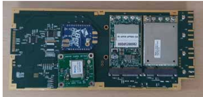
Fig. 4. Represents the generic PCB containing all replaceable modules (cellular in mini-PCIe form factor)
