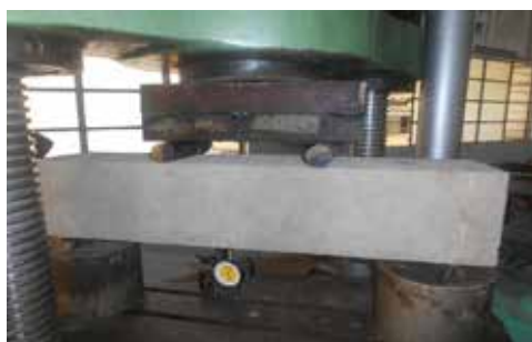
Figure 5. Testing arrangement of prism flexural strength
