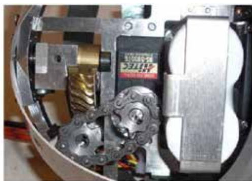
Fig 10. Roller chain connecting the servo motor to the worm gear
