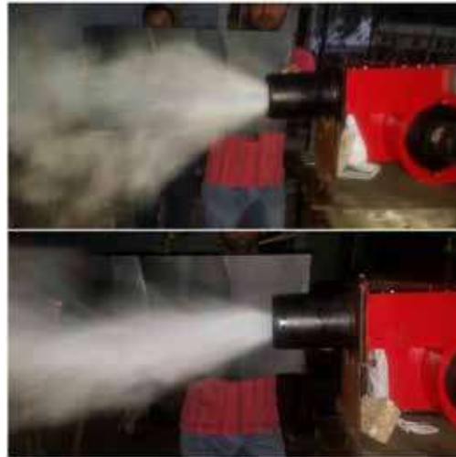
Fig. 3(a) Spray of fuel with different nozzle angle 60^\circ and 45^\circ respectively
