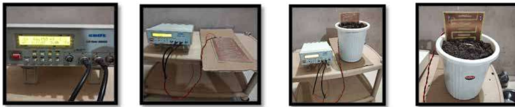
Fig. 6. Photographs of soil humidity measurement set up using IDC and RSFIDC
