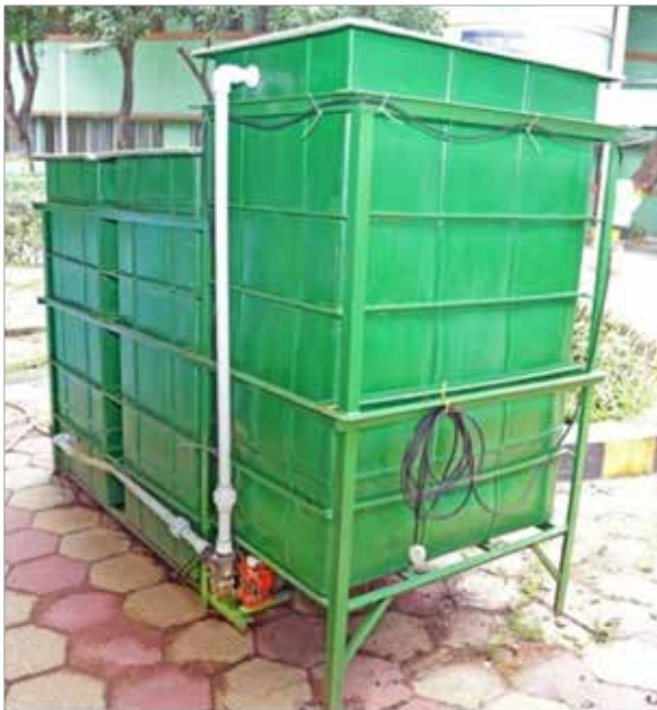
Fig. 3. Images of portable water tank for retting of jute ribbons and barky jute
