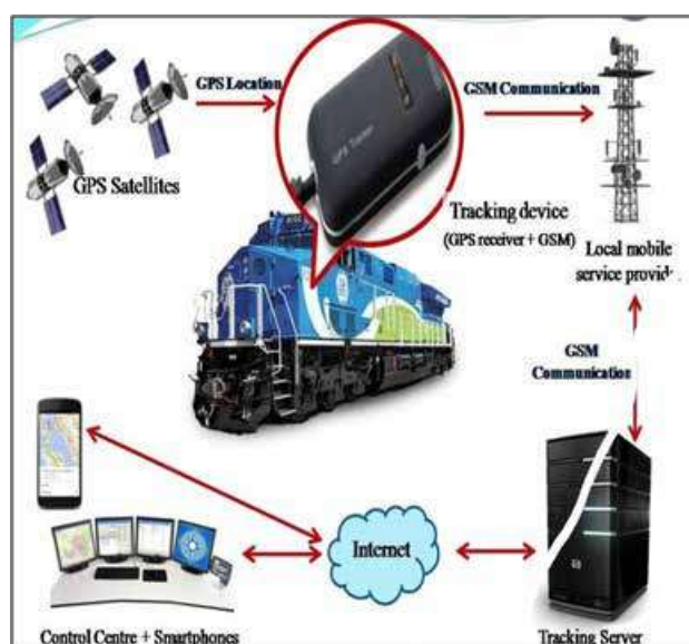
Fig. 1. Schematic of GPS / GPRS based vehicle tracking hardware
