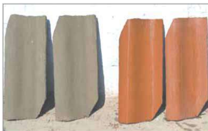
Fig. 10. Micro concrete roofing tiles produced using different blends of LC 3 [14]
