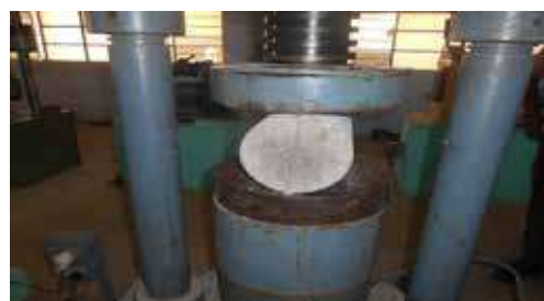
Figure 3. Testing arrangement of splitting tensile strength
