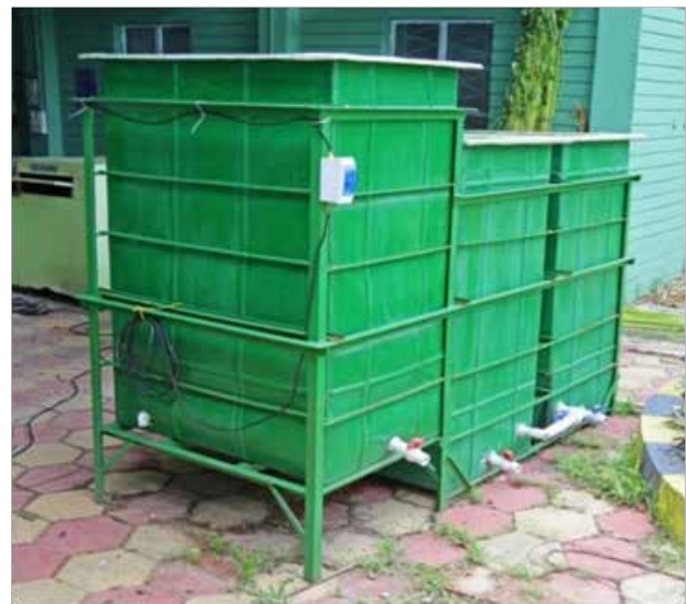
Fig. 3. Images of portable water tank for retting of jute ribbons and barky jute
