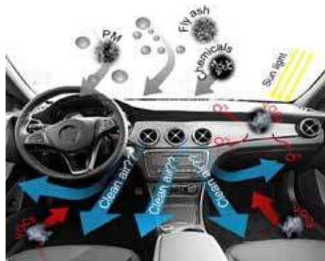
Fig. 1. The automotive cabin air filter removes harmful airborne pollutants and purifies cabin indoor air
