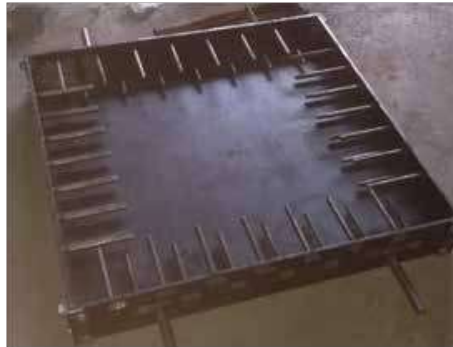
Fig.4. Slab specimen for restrained shrinkage test
