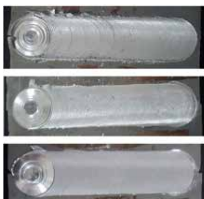
Fig. 2. Appearance of FS-Welded AA6061 alloy in (a) AC, (b) FWC, (c) UWC
