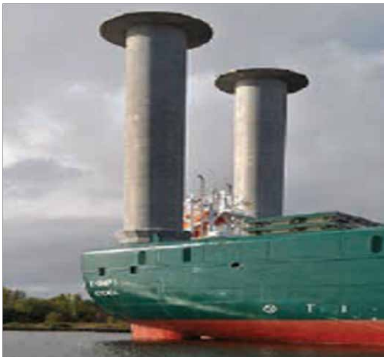
Fig. 3. Rotor sails, Flettner rotors are being developed. These utilize a so-called “Magnus Effect” for generating energy
