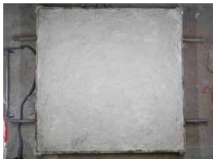
Fig. 6. Concrete specimen for early age shrinkage cracking test
