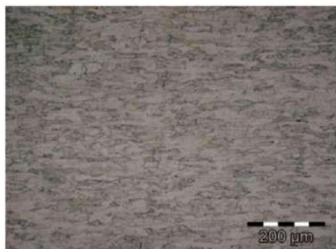
Figure 7 Optical Micrograph of hot rolled IF steel sheet X200
