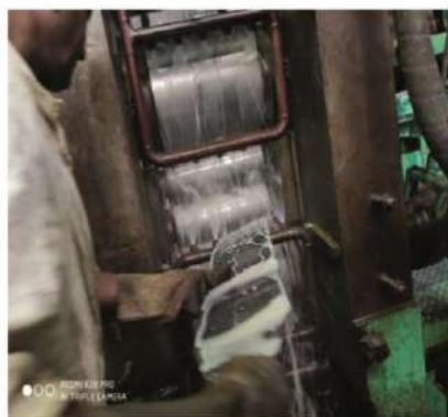
Figure 4 Experimental set-up (a) Rolling of IF grade steel at Experimental Rolling mill, RDCIS; (b) Muffle furnace for annealing, Kanthal Make.
