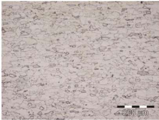
Figure 9 Optical microstructure of Cold rolled-annealed at 550^{\circ}\text{C} X200
