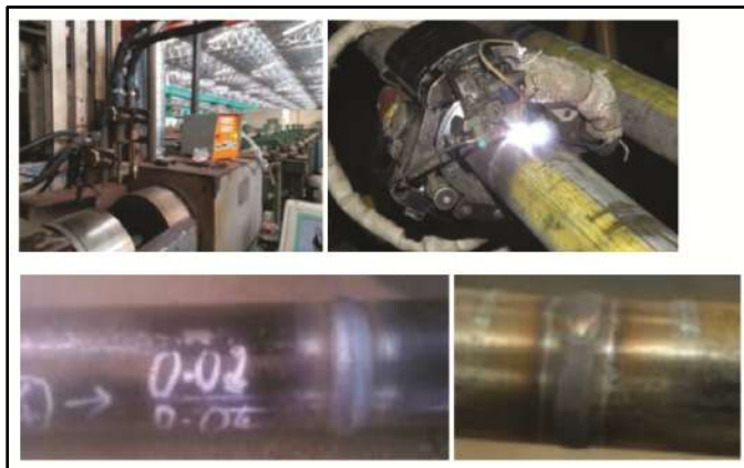
Figure 2 Set up & Weld Joint for A-GMAW process and ATIG processes
