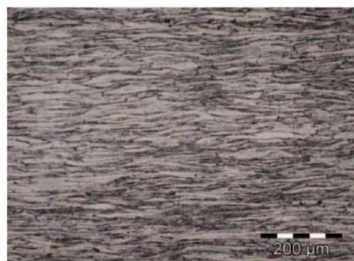
Figure 8 Optical microstructure of Cold rolled-Unannealed IF steel sheet X200
