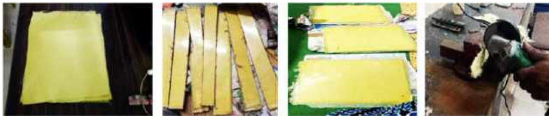
Figure 4 Preparation of tensile test specimens
