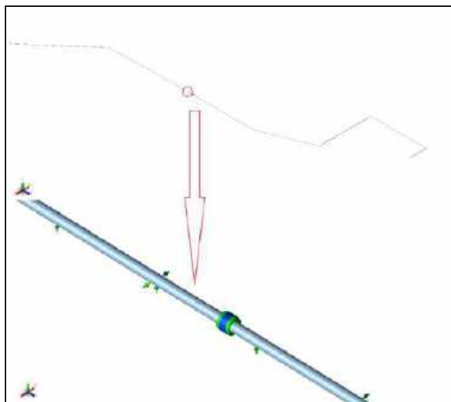
Figure 2 Pipe stress analysis model of COG pipeline, showing typical expansion joint installation
