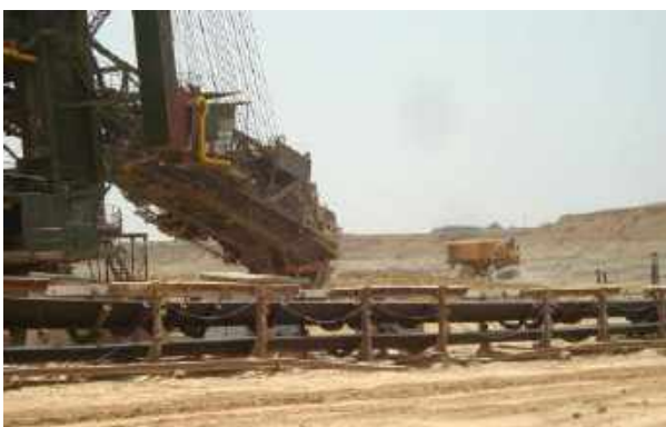
Photo 4 Dust emanation at Bucket Wheel Excavator in overburden cut face and controlled by continuous water spray arrangement
