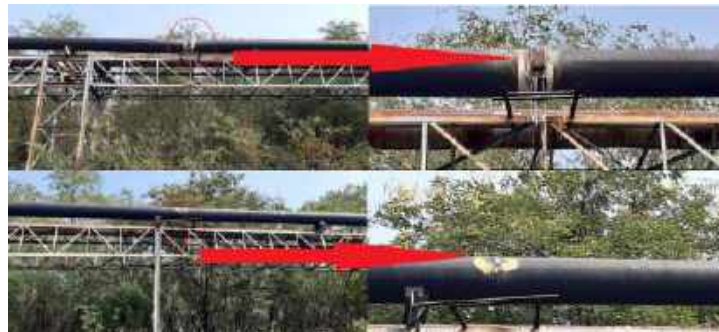
Figure 1 Failure of Circumferential Weld Joints of COG Pipeline
