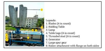
Figure 1 Various components of installed VAWT
