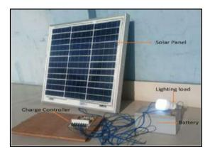
Figure 6 Experimental Setup
