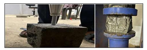
Figure 2 Rebound hammer test and Cube test of a typical concrete cube
