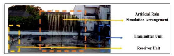
Figure 4 Artificial rain simulation setup
