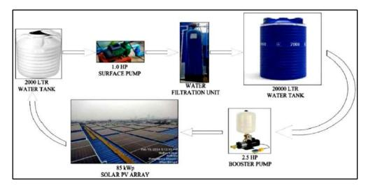
Figure 2 Cleaning-water recycling system for 85kWp solar PV power plant
