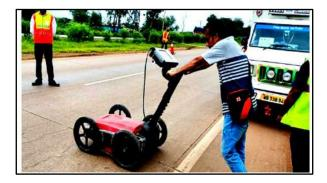
Figure 1 GPR Scan being conducted on the study stretch
