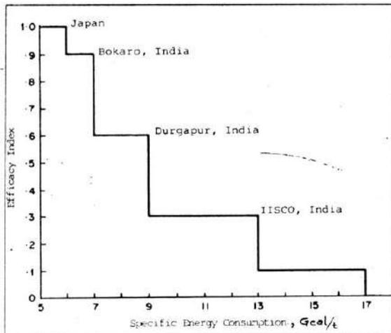
Fig 6 Efficacy index relationship for energy consumption in steel industry
