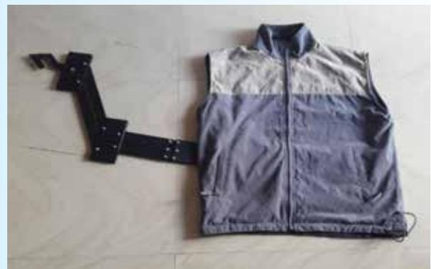
Final assembly of Carbon fibre frame with jacket (armour) front view
