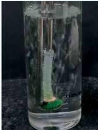
**Bubble column reactor for the integrated production of biosurfactant and Chromium metal recovery**
