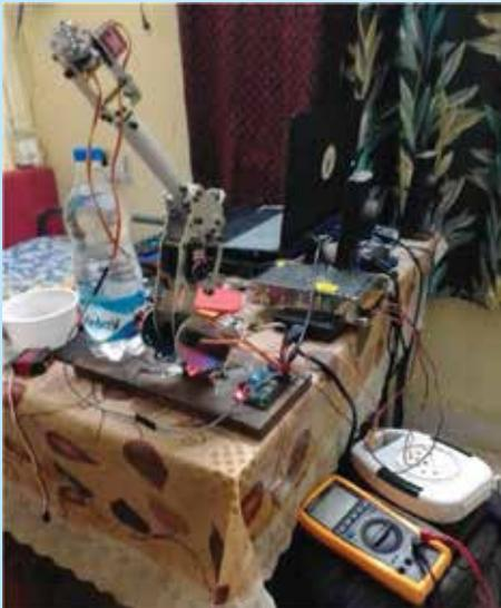
The Robot Arm Being Controlled via Internet
