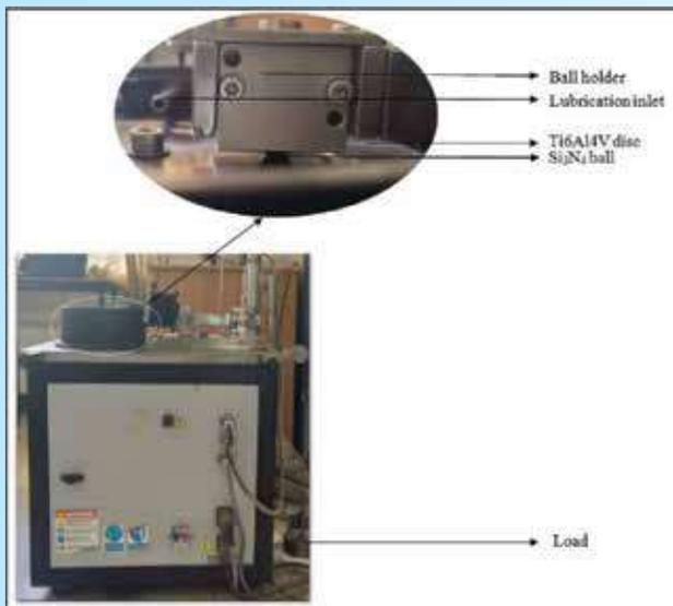
Modified Pin-on-Disc Tribometer
