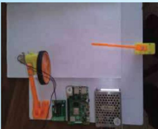
Fabricated Book reading system using 3D printing
