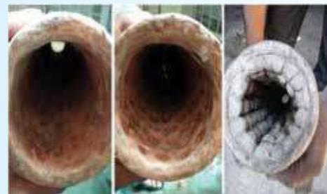
(a) Plane tube (b) Dimple Tube
