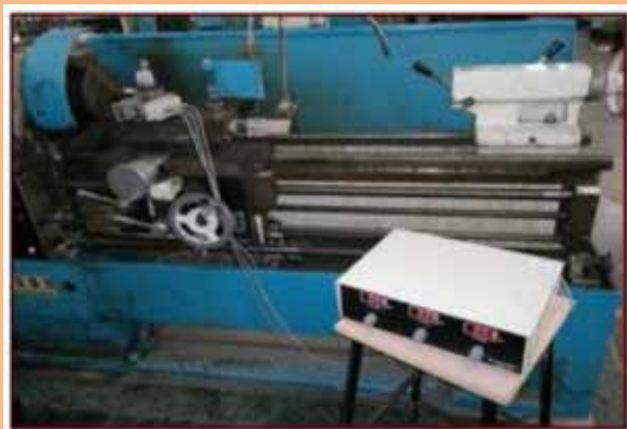
Force Dynamometer attached with Lathe during Experiment
