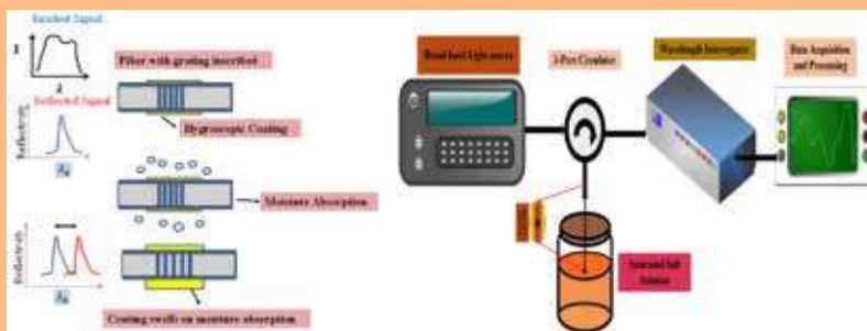
Figure 1: Hygroscopic behaviour and schematic of experimental setup
