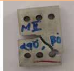
Broken piece shear loading
