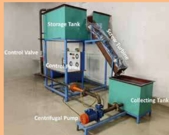
Final fabricated facility - Novel Screw Hydroturbine with Optimal Design
