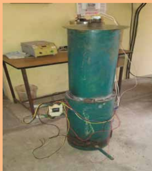
Fabricated setup of Pyrolysis Process
