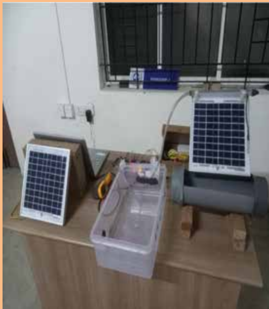
Schematic view of scaled solar PV/T system
