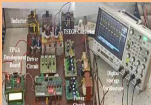
Laboratory Setup of TSEGS converter
