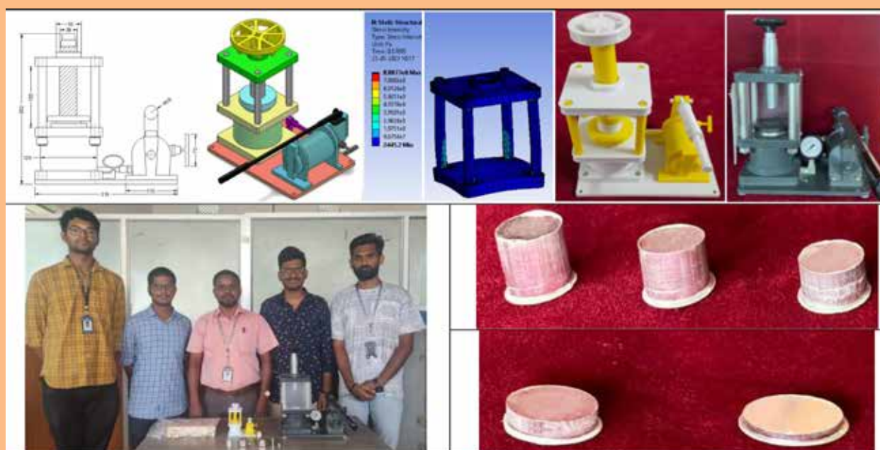
Design, Development and Fabrication of a 10 Tonne Portable Hydraulic Press for Powder Compaction
