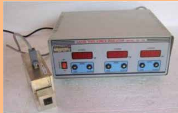
Lathe tool digital strain gauge dynamometer
