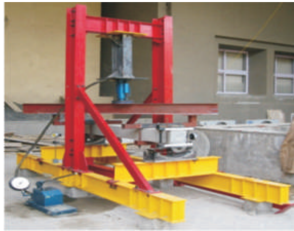
RC Beam subjected to combined bending and torsion in specially fabricated loading frame
