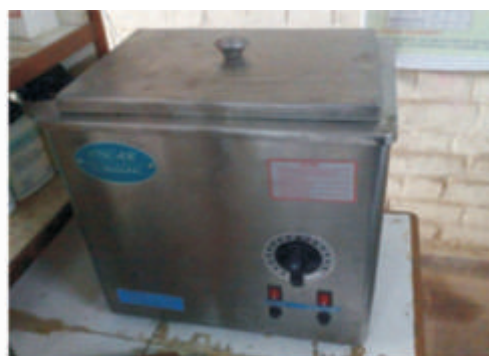
Ultrasonic bath (22 Hz, 120W) for degradation and scale up study of Rhodamine 6G
