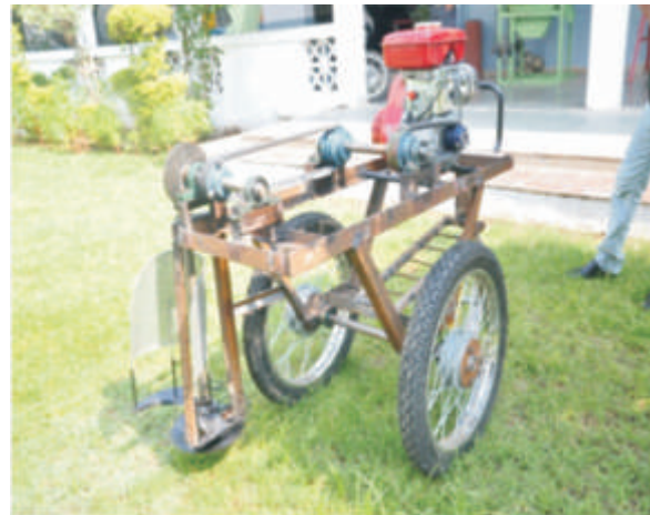
Wheat Ripping Machine at the time of testing at GHRCE lawn
