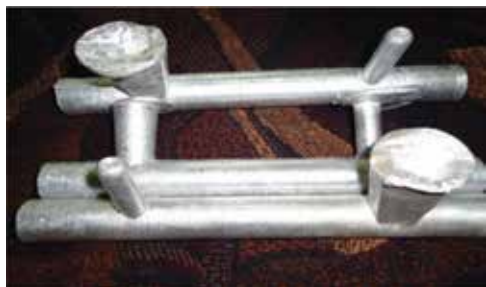
Cast Al/SiC/Al 2 O 3 Composite Rods
