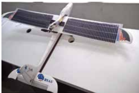
Solar Panel Fitted MALE Type UAV
