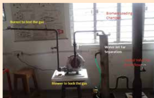
Biomass Gasifier with tar separator (Prepared)
