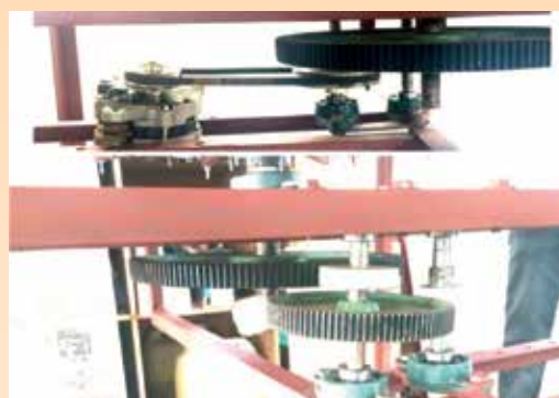
VAWT alternator with gear assembly
