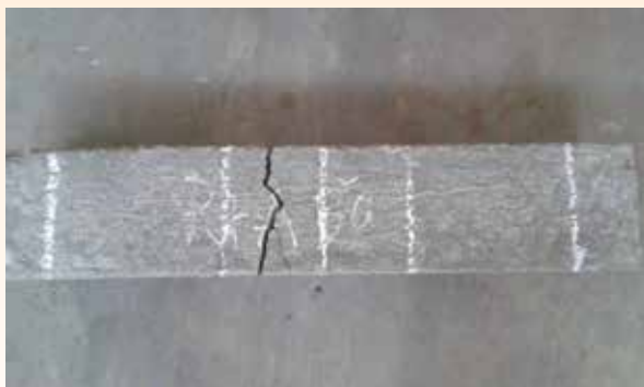
Failed specimens after flexure test
