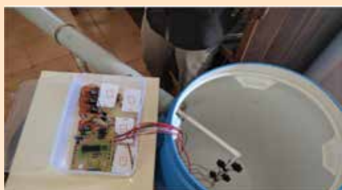
Gully pot monitoring system with integrated sensors
