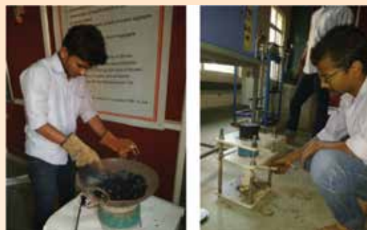
Preparation of mix and mould using flyash, plastic and bitumen with aggregates
