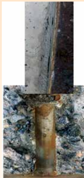
Adhesive bonded steel-concrete composite specimen connection interface failure
