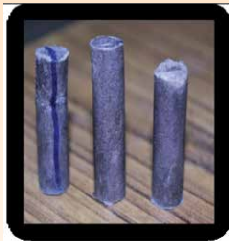
Pins prepared on FDM
