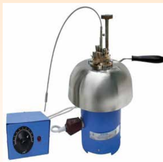
Experimental setup for measuring the Flash and Fire Point
