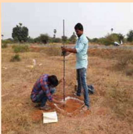
Cone Penetration test on reddish sandy soil in field
