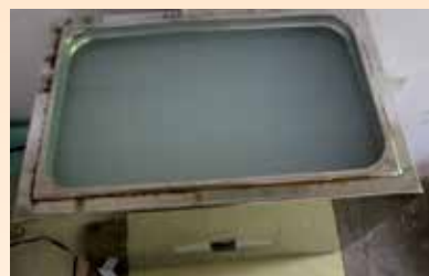
Prepared Nano-fluid through Ultrasonication
