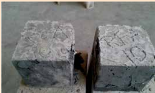
Failed specimens after compression test
