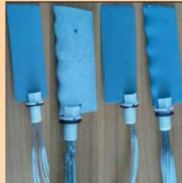
Normal and modified airfoils with pressure tappings
