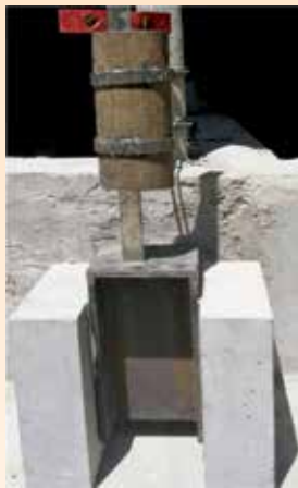
Adhesive bonded composite specimen subjected under drop weight impact test
