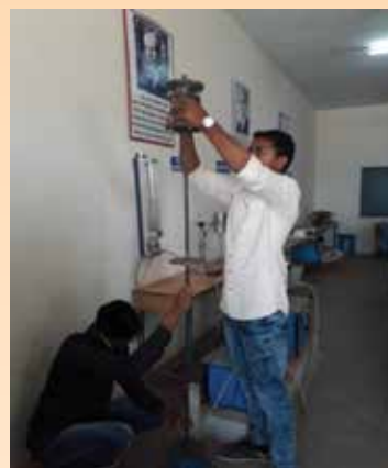
Cone Penetration test on blackish clay soil in lab
