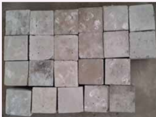
Geo-polymer concrete specimens cured at ambient temperature
