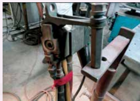
Plasma spray torch arrangement
