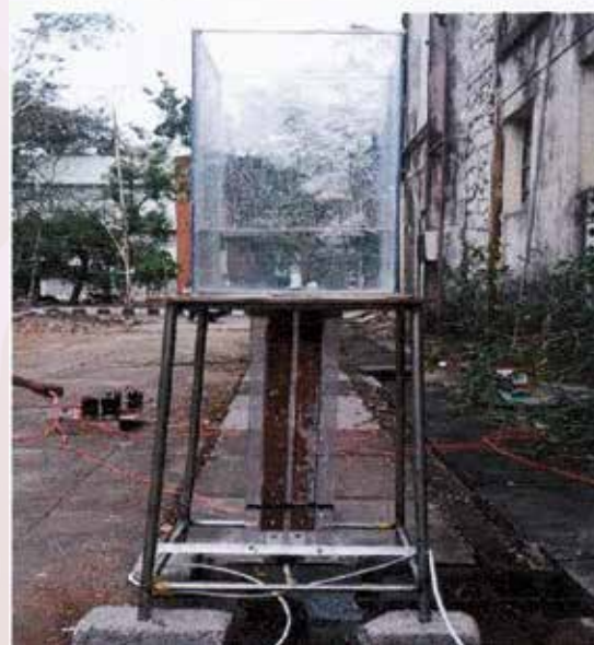
Projectile motion in the rails (captured and processed with image processing tools) scaled underwater launcher setup
