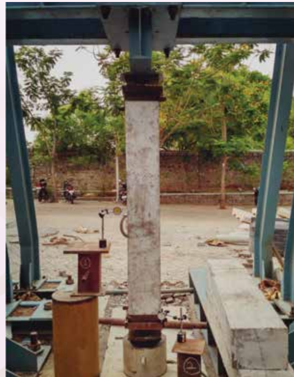
Experimental test set up for column with EOF steel slag as aggregate
