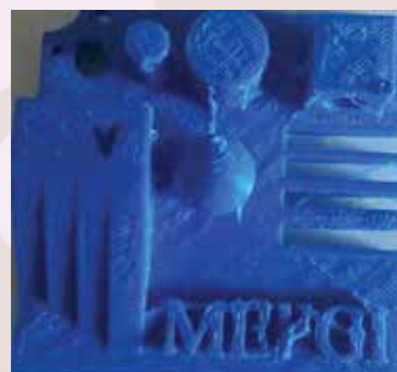
Specimen printed with ABS – variable slicing
