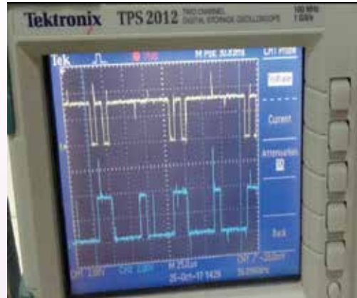
PWM pulses of inverter (T1 and T2) with maximum shoot through
