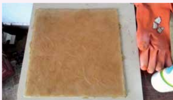
Composite Plate – Microfibrillated fiber / Polyester matrix
