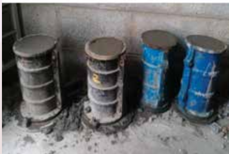
Casting of specimens to study primary properties of concrete
