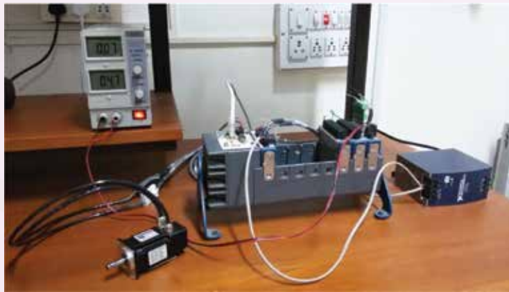
Experiment set up – Compact RIO, drive, I/O module and motor
