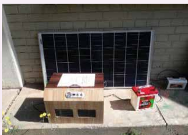
Complete Portable Solar Refrigerator with Solar Panel and Charge Controller
