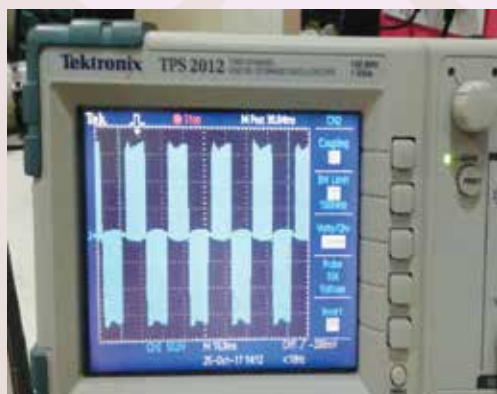
Output voltage of the Inverter with maximum shoot through (170V)
