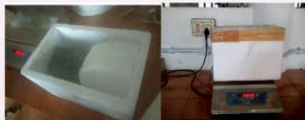
CO 2 adsorption test using dry ice
