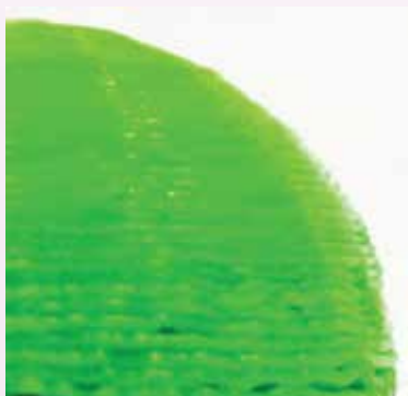
Hemisphere built - variable slicing, side view
