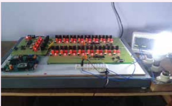
Cascaded H Bridge Multilevel Inverter Hardware setup (without solar panel)
