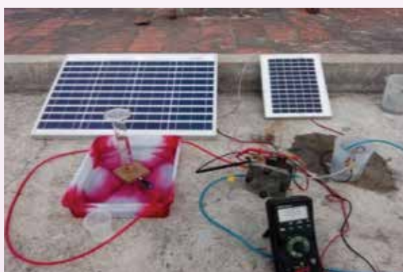
Final Experimental Setup for Optimize Direct Coupling of Solar PV with PEM Electrolyser
