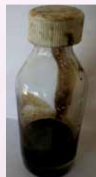
Fuel oil produced using the designed set up from e waste
