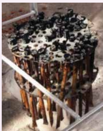
SiO 2 coated NaNO 3 pellets are inside copper tubes
