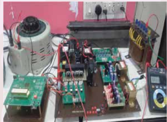
Z-source Inverter connected to 500Ω and 25 mH resistive, inductive load
