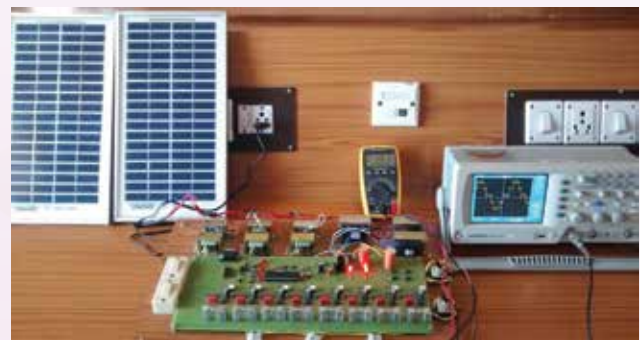
Cascaded H Bridge Multilevel Inverter Hardware setup (with solar panel)
