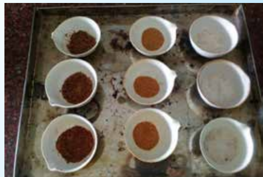
Determination of organic content in soil samples using ASTM method
