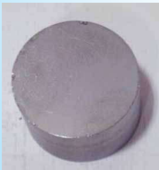
Germanium Ingot, 99.999% purity, 1 in. diameter and 0.5 in. Tall
