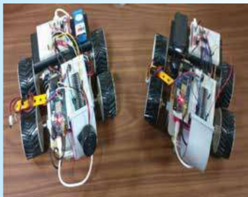
Vehicles with the 'Intelligent Collision avoidance System using IoT' is implemented using Raspberry Pi 3
