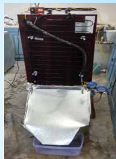
Mist cooled condenser arrangement in domestic refrigerator with Pressure and Temperature measurement system
