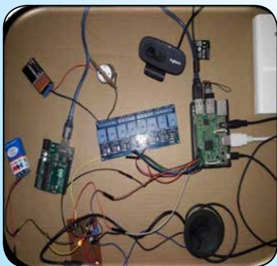
Personal Assistant to Control Fan and Light Using Raspberry Pi with Voice
