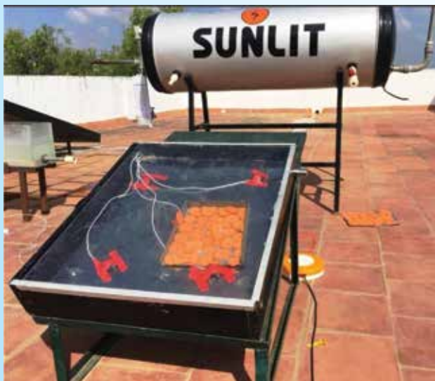
Schematic view of experimental setup with as a dryer unit
