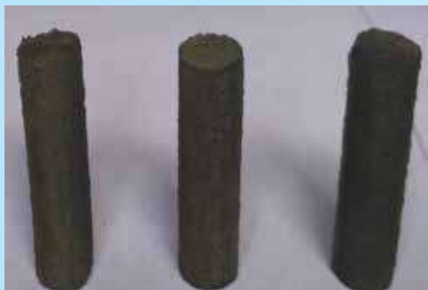
specimens of Ti-6Al-2Sn-4Zr-2Mo
