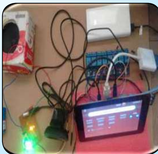
Personal Assistant to Control Fan, Light, AC and PPT using Raspberry Pi with LCD Touch Screen
