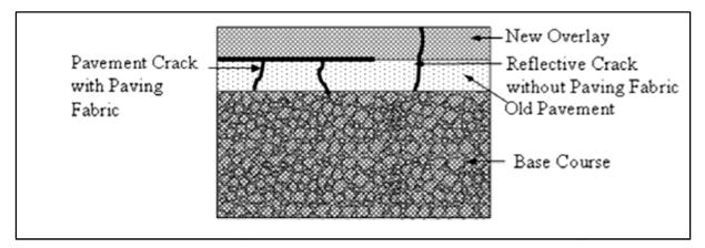
Figure 1 Application of Strain Absorbing Membrane Interlayer (SAMI)
