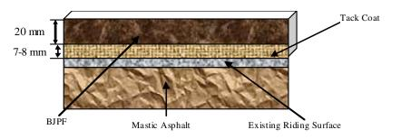
Fig. 1 Sectional View of the Design of the Field Trial with the Developed BJPF
