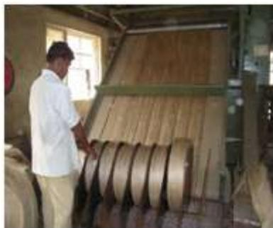
Photo 1: Feeding of the carded slivers for Nonwoven Fabric preparation
