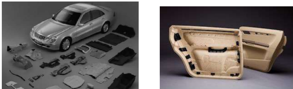
Fig.4 Components made by natural fibers for Mercedes-Benz E-Class components (source: Sue Elliott-Sink, 2005)
