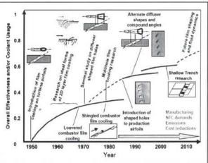
Gas Turbine Film Cooling e modern turbine inlet temperatures exceed the melting
