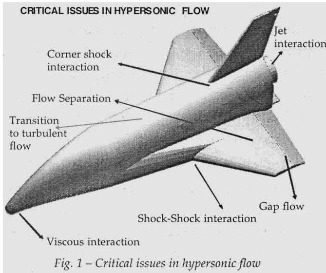
Both experimental and numerical simulations play a significant complementary role in hypersonic vehicle design. Basic experimental studies are required to understand the physics, and also to get sufficient data to enable the designer to model the phenomenon.
