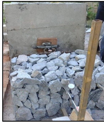
Figure 1 A typical testing setup for gabion wall
