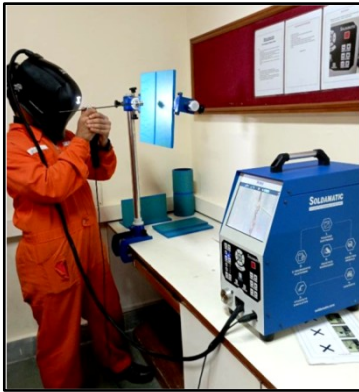
Figure 1 B. Tech Engineering trainee performing Single Butt Joint (3G) welding using Augmented Reality welding Simulator (Tolani Maritime Institute)
