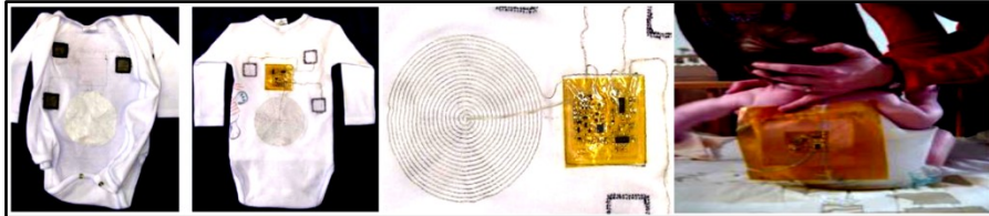
Figure 2 Baby suit prototype. Left: inside showing the Textrodes; right: backside, Detail of the backside of the baby suit, showing the embroidered coil and the flexprint, Demo set-up with belt prototype, worn by a 12 weeks old baby [18]
