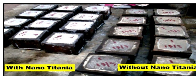
Figure 4 Casted Nano Titania (NT) Cementitious Composites (left) and Reference Specimen (right)
