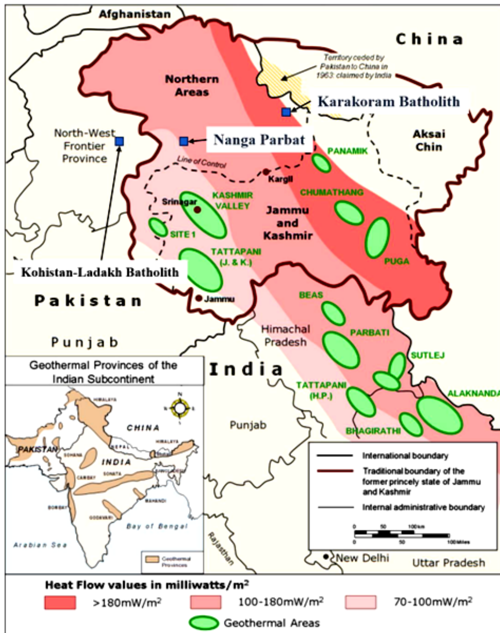
Figure 1 Geothermal provinces of the Indian subcontinent, highlighting heat flow values across regions and key geothermal areas. The red shaded areas indicate varying levels of heat flow ( \text{mW/m}^2 ), with the highest values ( >180 \text{ mW/m}^2 ) observed in the northern regions, including Kohistan-Ladakh Batholith, Nanga Parbat, and Karakoram Batholith. Green ellipses mark significant geothermal sites in India.
