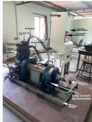
Figure 1 VCR test engine
