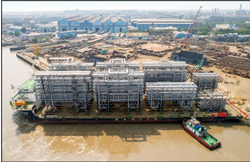
Photograph 2 Modular plant being transported, at loading port of LTEH, Hazira
