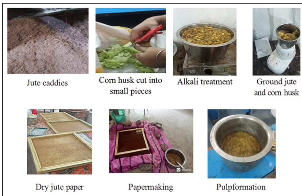
Figure 2 Flowchart of papermaking from jute caddies and corn husk
