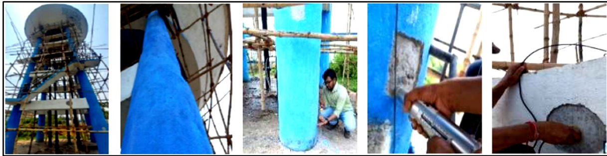
Figure 1 (a)-(b) Real-life RCC OHR subjected to constructional imperfection, (c)-(e) visual inspection & non-destructive tests
