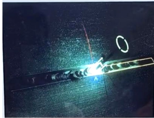
Figure 2 The screen image seen through the headset (SOLDAMATIC Augmented Reality Simulator)
