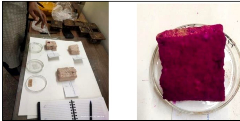
Images 4A & 4B Carbonation testing of lime mortar executed
