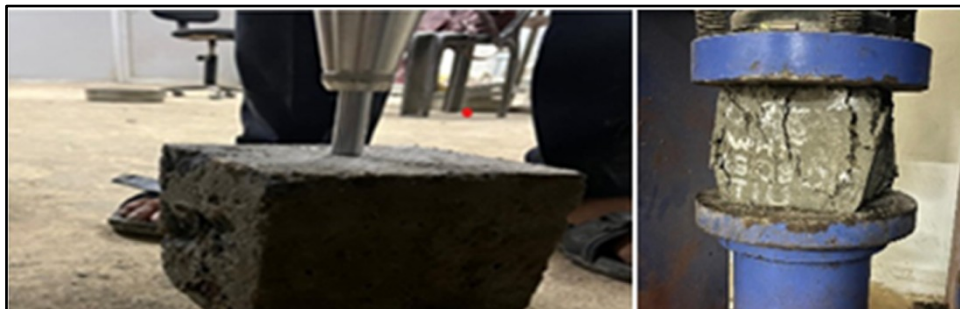
Figure 2 Rebound hammer test and Cube test of a typical concrete cube
