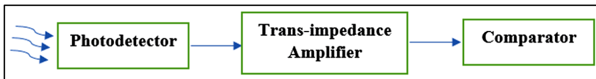
Figure 2 Illustration of Receiver Element of the emblematic FSO Arrangement
