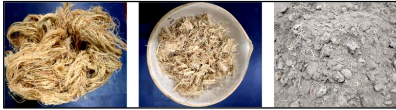
Figure 1 Water hyacinth fiber and concrete mix
