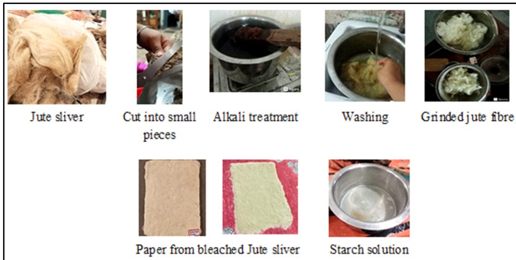
Figure 1 Flowchart of papermaking using jute sliver
