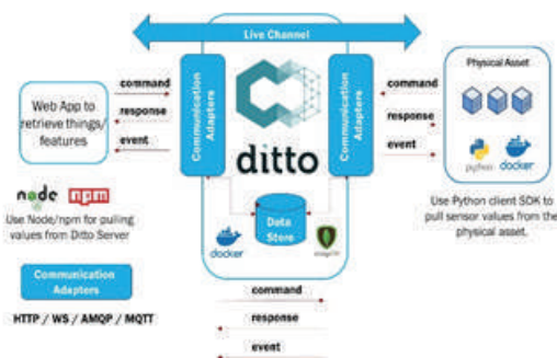
Fig. 3. A digital twin system using Eclipse Ditto
