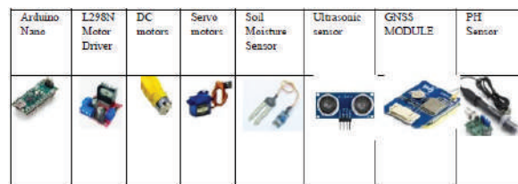
Fig 2: The components that are used in this autonomous robot
