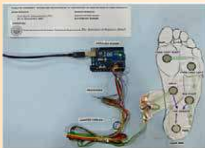
Experimental setup of the foot pressure measuring system
