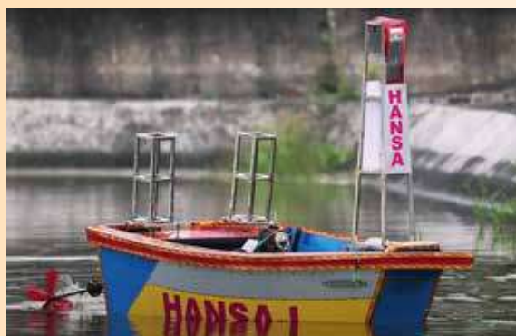
Fig. 1 Front view of Hansa 1: Unmanned Surface Vehicle made for water surface pollution monitoring
