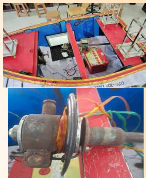
Fig. 2 Top view and propeller driver unit of Hansa 1
