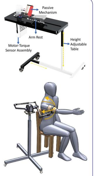
Fig. 7 : Device for (a) Hand neurorehabilitation and (b) Arm neurorehabilitation
