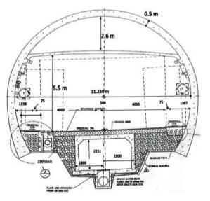
Figure: Cross section of the tunnel
