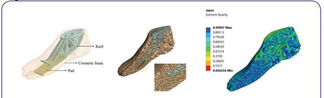
Fig. 8 : Geometry of a solid Ankle cushioned heel (SACH) foot from 3D scanning and processing and its corresponding meshed finite element model
