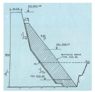
Figure: Section of Strengthened Koyna Dam after 1967 Earthquake
