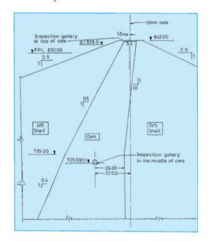
Figure: Mid-level Inspection gallery & Top Level Inspection Gallery in Dam Section
