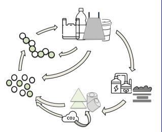
Fig. 1 : Schematic overview of a circular plastics economy, which involves shifting production from fossil to renewable feedstock including biomass,  $CO_2$ , etc., design of plastics to possess features for mechanical or chemical recycling, and alternatively recycling the carbon by biodegradation in a controlled environment.
