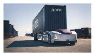
Fig. 10 : Self driving truck from Volvo
