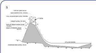
Figure: Cross-sectional view of the Sardar Sarovar Dam
