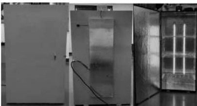
Fig 6: Fabricated UVC sterilization chamber (front view, rear view, UVC and rack arrangement)
