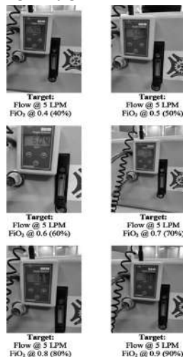
Fig 7: Variations of a \text{FiO}_2 with 5 LPM through Manual Control
