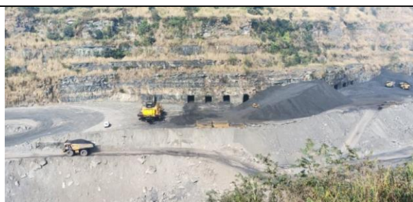
Figure 2: Photograph showing web cut and web pillars in highwall mining at West Bokaro Mine.
