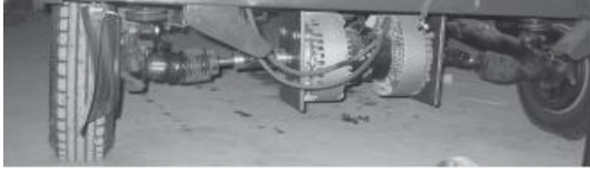
Fig. 4 Two Etek motors mounted on the autorickshaw readily available in India.
