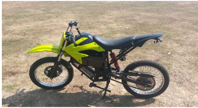
Fig. 4: A prototype of an off road electric bike
