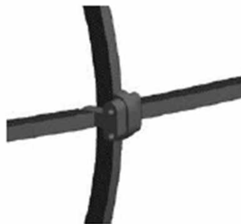
Figure 2 : CAD model: Sandwich joint
