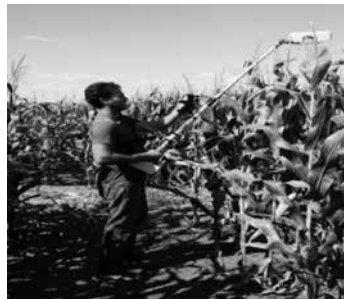
Collecting NDVI data using the Trimble® GreenSeeker® crop sensing system
