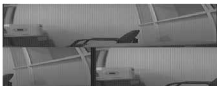
Figure 5 : Packed YUV interlaced frame
