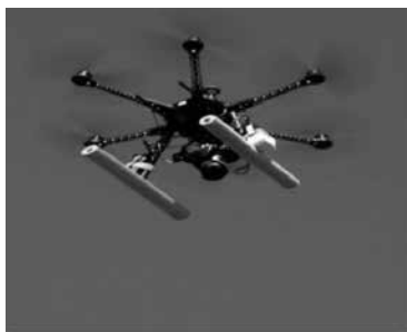
Collecting color infrared imagery using Hexcopter and Canon T4i NDVI camera
