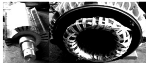
Figure 12(b) : Fabricated rotor and stator assembly of BDFRM
